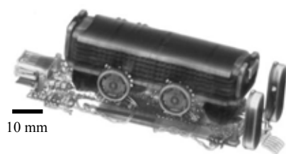
Figure 1 Volume rendering of a commercial UPP fuel cell (Intelligent Energy) - a device used for charging of portable electronics
