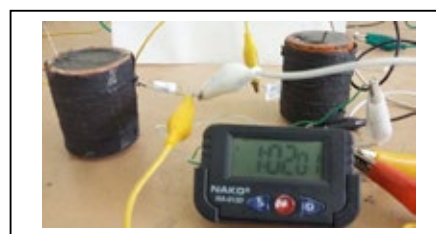
Fig. 1. AV-C-MFCs powered digital clock
