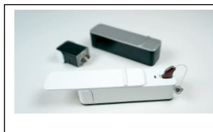
Fig. 1. DMFC powered hearing aid and refueling station.
