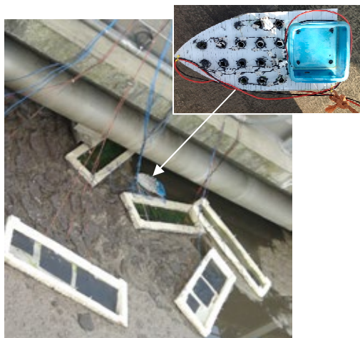
Fig 1. Floating plate microbial fuel cells in the anoxic tank of wastewater plant Milano-Nosedo. Inset: boat-shaped floating system with 16 terracotta MFCs.
